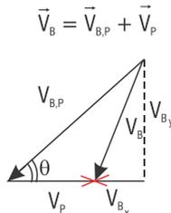
$$V_B^2 = V_{Bx}^2 + V_{By}^2$$
