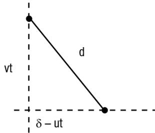
$$d^2 = v^2t^2 + (\delta - ut)^2 = v^2t^2 + u^2t^2 - 2\delta ut + \delta^2 = (v^2 + u^2)t^2 - 2\delta ut + \delta^2$$
